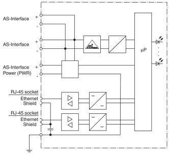
At the cable for power supply no slaves or repeaters may be attached.
